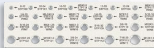
Figure C.2 Use the Thread Sizing Board to determine the thread size of the IM nail cap. Use the size measurement to select the appropriate threaded extractor tip
